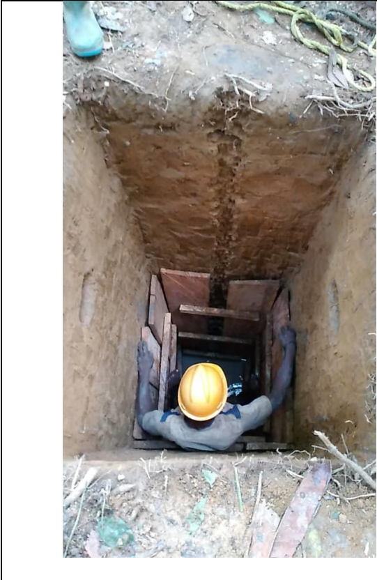
Channel sampler in pit
