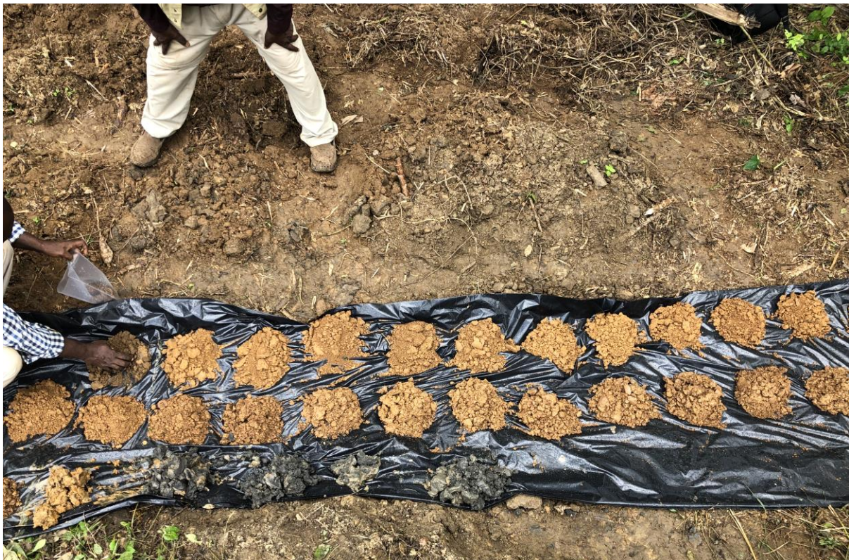
Figure 14.1: Nkoteng BWA_Deane_Loc2e_DH039 twin auger sample profile
