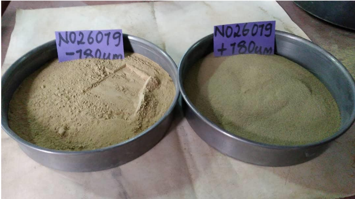
Figure 14.5: Separation of fractions from sample N026079.
